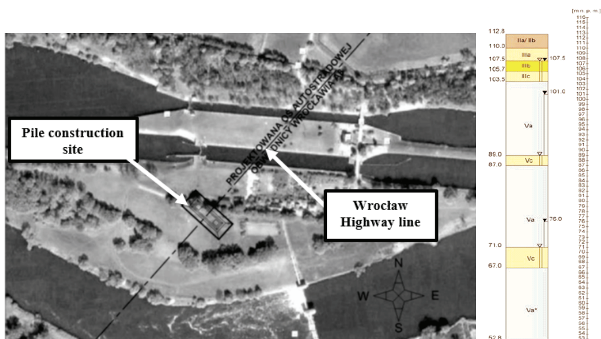
Fig. 2. Construction site and soil profile [2]
