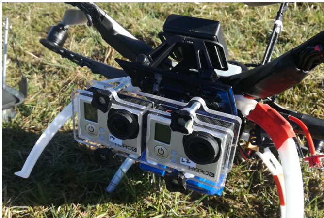
Fig. 1. Stereo rig with GoPro cameras mounted on tested MAV
