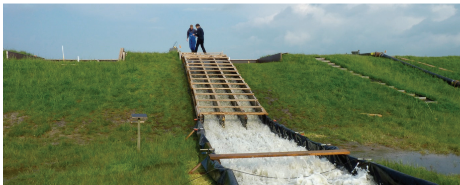
Fig. 7. Flume setup on the Rostock research dike
