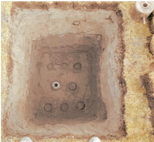
Fig. 4. Sample of bottom ash – dredged sand mixtures obtained from excavation
