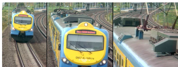
Fig. 8. Set of three camera images taken, for identification of vehicle and raised pantograph
