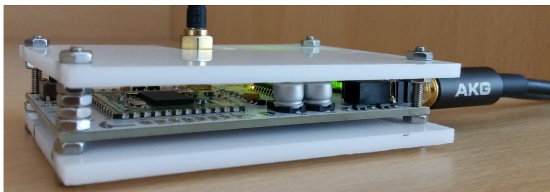
Fig. 5.10. Operating programmable DAB+ receiver.
