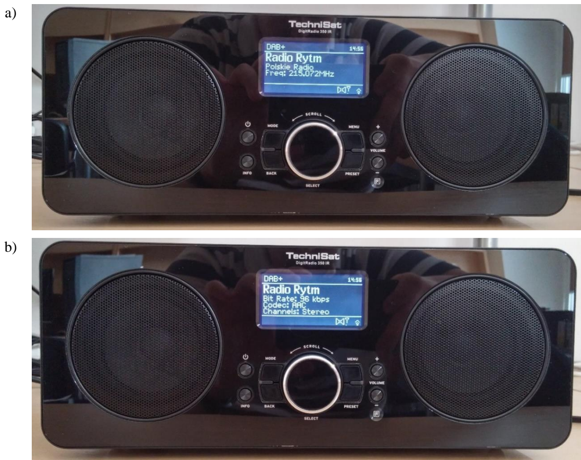
Fig. 5.12. TechniSat DigitRadio 350 IR receiver: a) frequency info, b) bitrate info.
