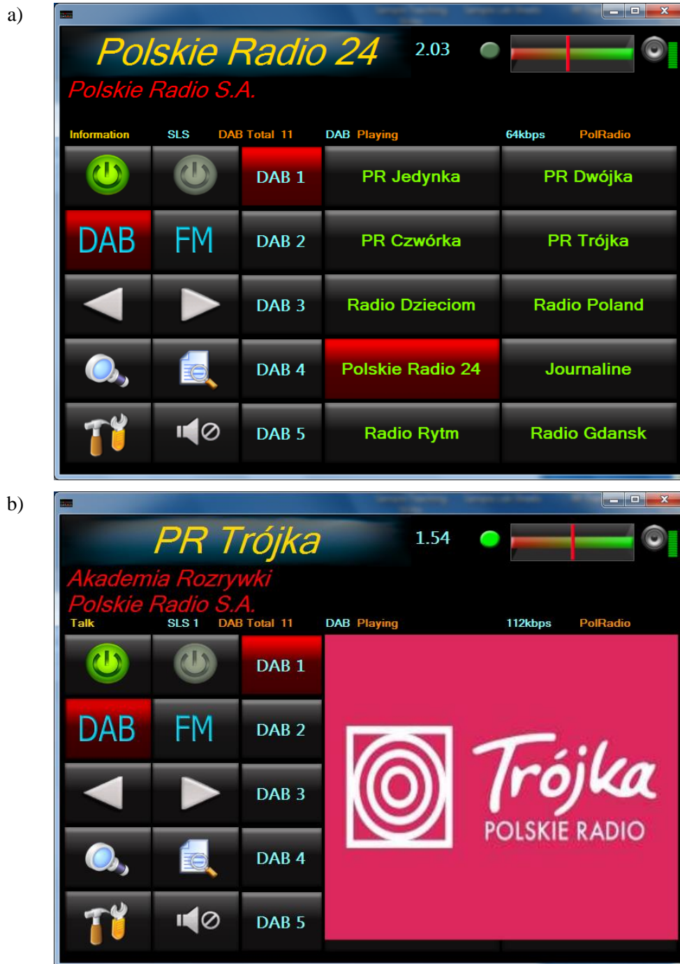
Fig. 5.11. DAB+ programmable receiver GUI user interface: a) main menu, b) SLS menu.
