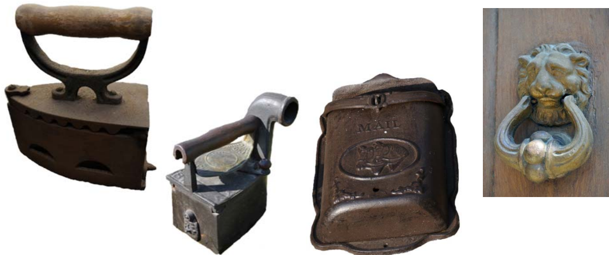
Figure 2. Cast iron irons with holes assuring the inflow of oxygen into the device with burning embers inside. On the left example: semi-circular holes on sides; on the right example: the hole in shape of pipe above the handle and a metal plate protecting hand from high temperature
