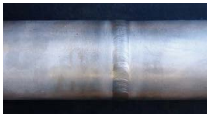
Fig. 4. Test joint no. 1 viewed from the weld face side; the specimen was subjected to cleaning and passivation
