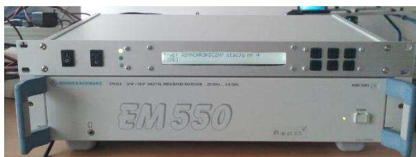
Fig. 4. Base station prototype: dedicated transmitter (top) and commercial receiver (bottom) [authors' photos]
