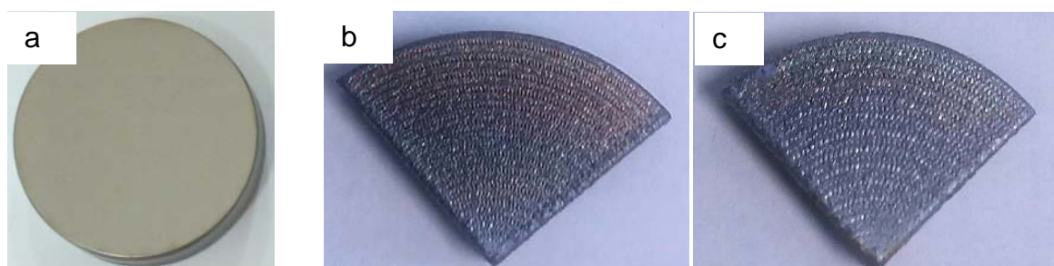
Fig. 1. Surface microstructure of the Ti13Nb13Zr alloy: a) before laser treatment and cut (BM) b) after laser treatment (LT 1), c) after laser treatment (LT 2)
