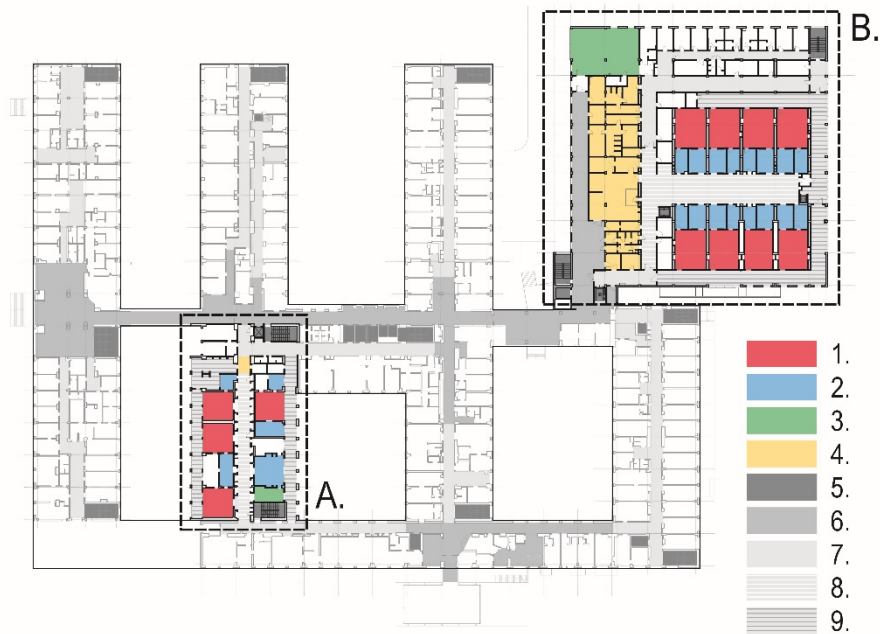
Figure 1: Comparison of the size and the spatial arrangement of the operating theatre. Voivodship hospital in Elbląg, before (A) and after expansion (B). Explanatory figure, a former operating theatre was located on the ground floor, the new one on the 1st floor. 1 = operating rooms, 2 = patients and staff preparation rooms, 3 = post-operation rooms, 4 = patients, staff and material locks, 5 = staircases and lifts, 6 = general hospital communication, 7 = in-wards communication, 8 = internal clean route, 9 = internal dirty route. Project by. arch. S. Sosak, 2012.
