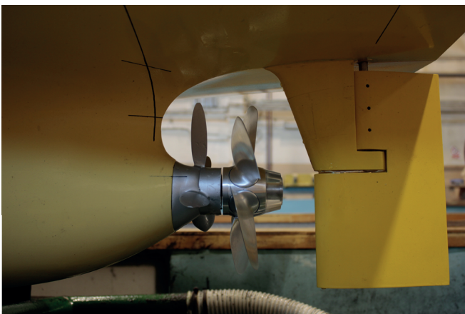
Fig. 6. Self-propulsion test arrangement with pre-swirl stator
