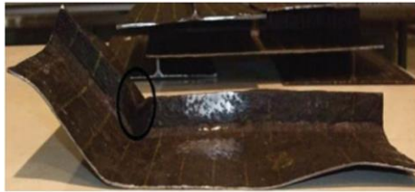
Figure 14: Tested [7] (left) and simulated (right) post-collapse shape of specimen 1.
