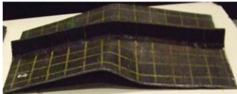
Figure 16: Tested [7] (left) and simulated (right) post-collapse shape of specimen 3.
