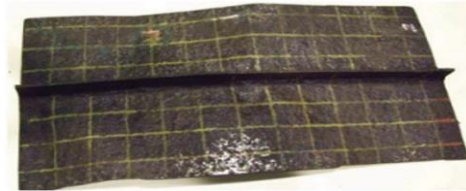
Figure 15: Tested [7] (left) and simulated (right) post-collapse shape of specimen 2.
