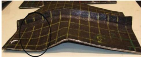
Figure 17: Tested [7] (left) and simulated (right) post-collapse shape of specimen 4.
