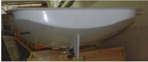
Fig. 10 Model with appendages during the test
