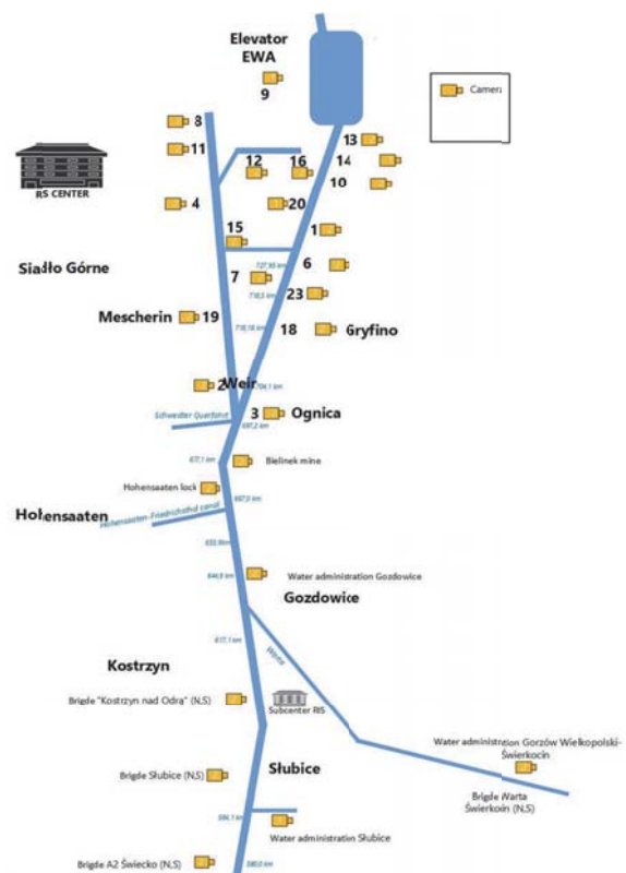
Fig.1. Schema of existing and planned cameras on Odra RIS area. [own elaboration based on 5]
