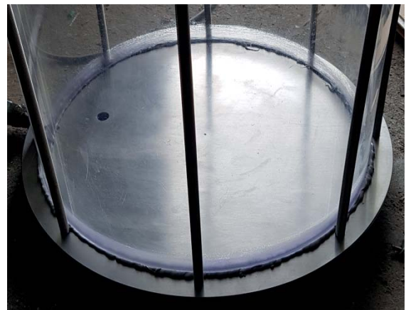
Fig. 8. Sealing of lower tank
