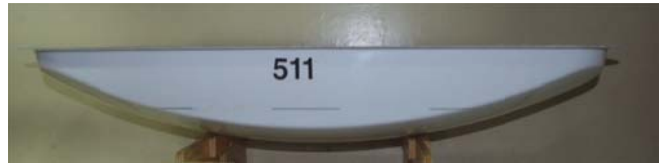
Fig. 5 Side view of the model without appendages
