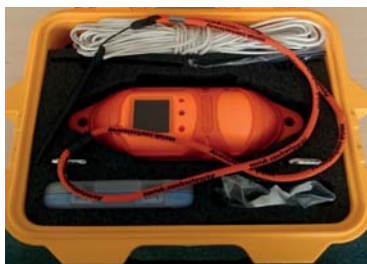
Fig. 11. Sonic sounder for measuring sound speed
