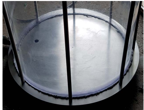
Fig. 8. Sealing of lower tank
