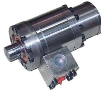
Fig. 1. General view of PSM-0,75 pump
