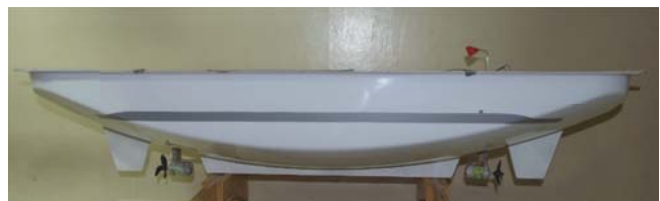
Fig. 7 Side view of the model with appendages
