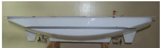
Fig. 7 Side view of the model with appendages
