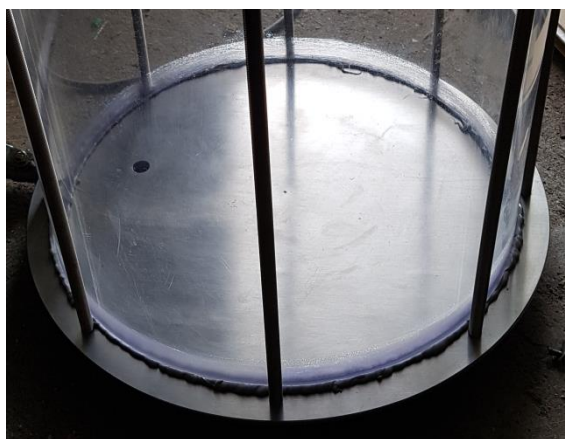
Fig. 8. Sealing of lower tank
