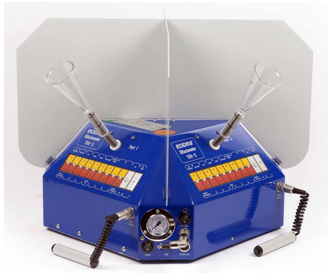
Figure 4. Example of a dynamic olfactometer
