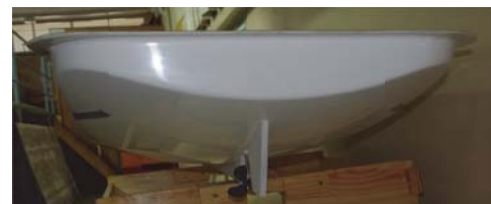
Fig. 9 Model without appendages during the test
