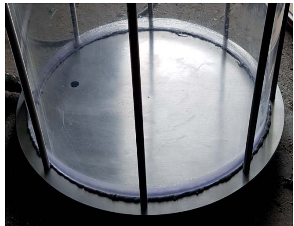
Fig. 8. Sealing of lower tank
