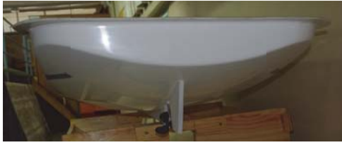
Fig. 10 Model with appendages during the test
