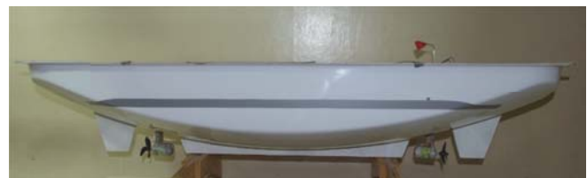
Fig. 7 Side view of the model with appendages
