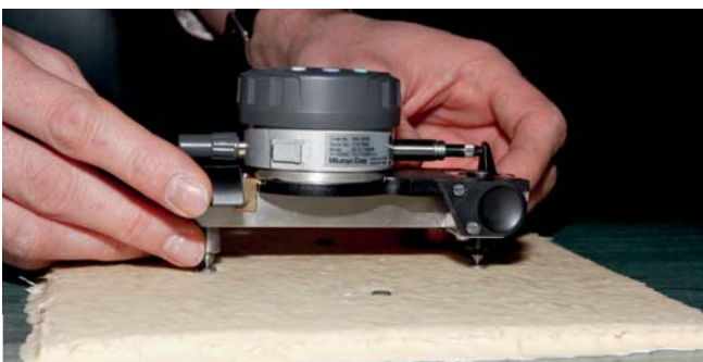
Fig. 5. Extensometer used for length change measurement
