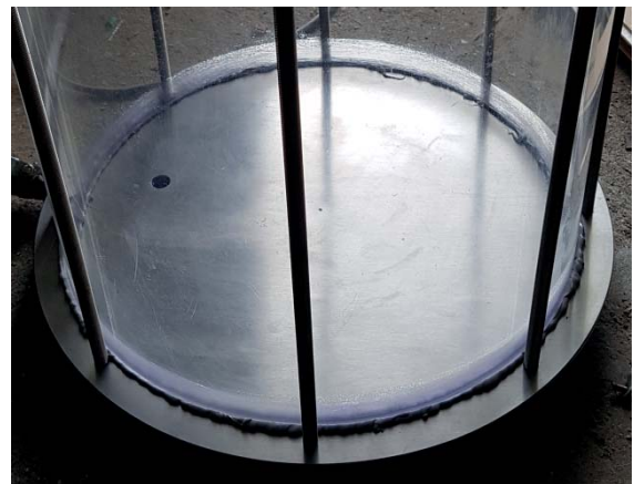
Fig. 8. Sealing of lower tank
