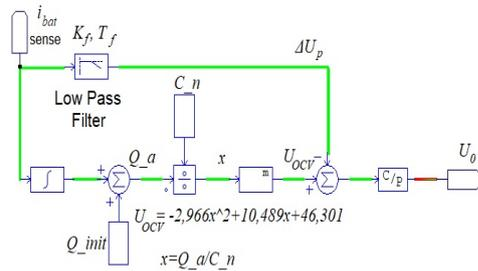
Fig.1. Mathematical model of AHF battery;
