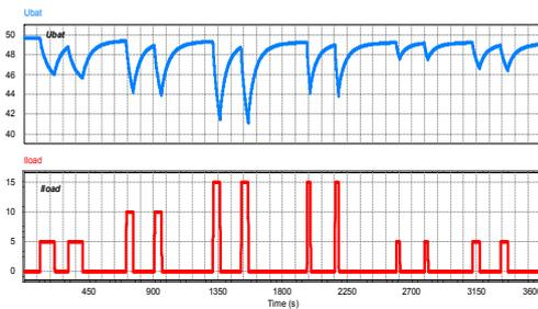
Fig.9. Voltage  $u_{bat}$  variation of the hybrid storage forced by pulse current profile  $i_{load}$  (Pulse Width  $2 \times 100 \text{ s}$ ,  $2 \times 50 \text{ s}$ ,  $2 \times 50 \text{ s}$ ,  $2 \times 25 \text{ s}$ ,  $2 \times 25 \text{ s}$ ,  $2 \times 50 \text{ s}$ )
