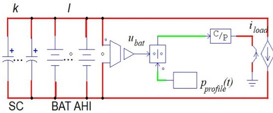
Fig.14. Hybrid storage with simulated load  $i_{load}$  based on power profile  $p_{profile}(t)$  for  $t \in <0, T>$ .  $T$  is the time, at which the hybrid storage is loaded
