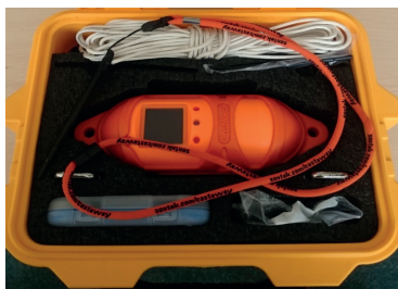
Fig. 11. Sonic sounder for measuring sound speed
