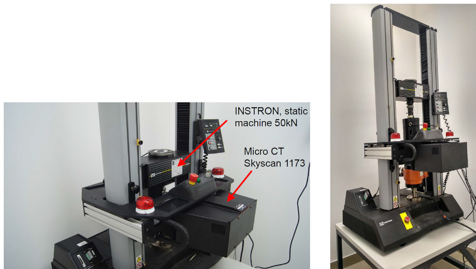
Fig. 13. Micro-CT Skyscan 1173 mounted on an Instron 5569 quasi-static machine.
