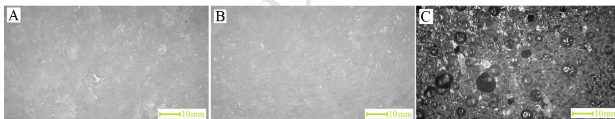
Fig. 12. Sample images of the surface topography after fracture for the tested specimens: A) unmodified bone cement, B) antibiotic-loaded bone cement and C) bone cement modified with nanometals (LM - mag. 30x)
