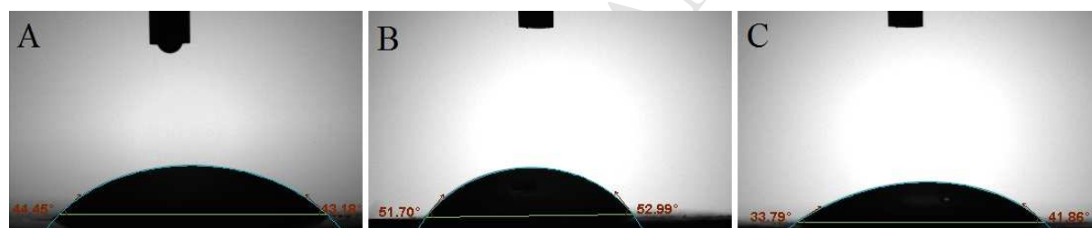
Fig. 6. Sample measurements of the contact angle for the tested specimens: A) unmodified bone cement, B) antibiotic-loaded bone cement and C) bone cement modified with nanometals
