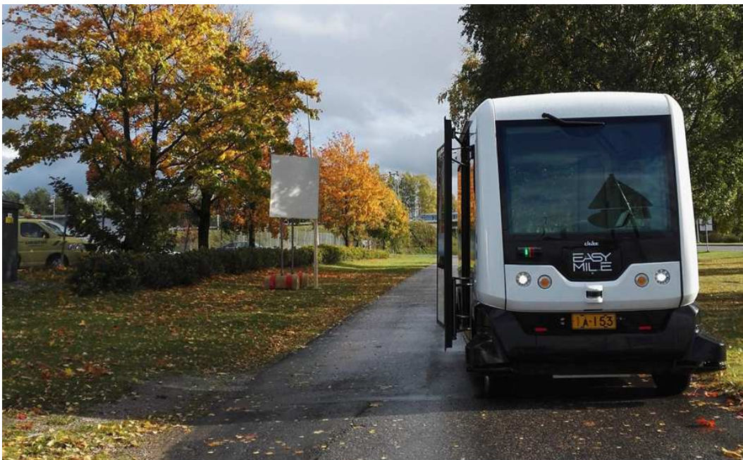
Figure 14. Localization signs were needed on the Helsinki route, there were not enough fixed structures in the end of the path.
