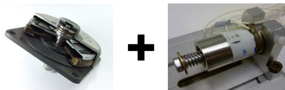
Fig. 1. The ultrasonic traveling wave motor [15] and rotating mode motor [16].
