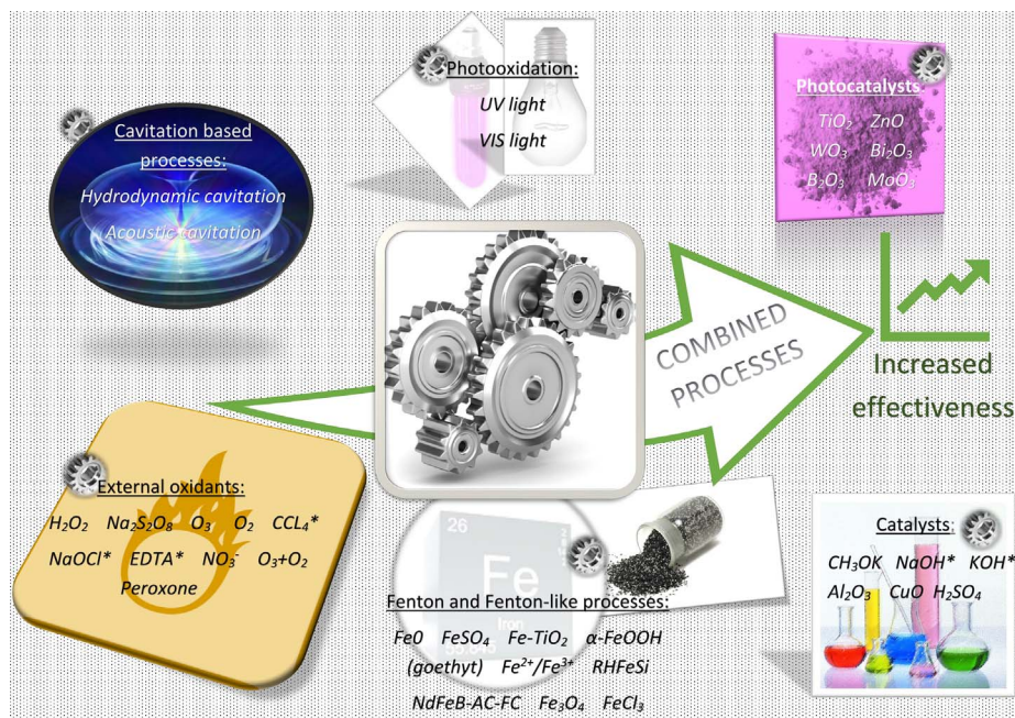
Fig. 3. Cavitation in combination with AOPs in wastewater treatment processes. EDTA – was found to break down O–O bond of oxygen and produce \text{H}_2\text{O}_2 in a Fe/EDTA system [94]; NaOCl – commonly known as bleaching agent, is frequently used as a disinfectant for treating drinking water [135]; \text{CCl}_4 – as a hydrophobic organic compound, is prone to enter the cavitation bubbles and undergoes degradation by pyrolytic cleavage to produce large amount of Cl radicals [85,123,137]; NaOH and KOH – used as alkaline catalysts in combined process with hydrodynamic cavitation for methane production [65].
