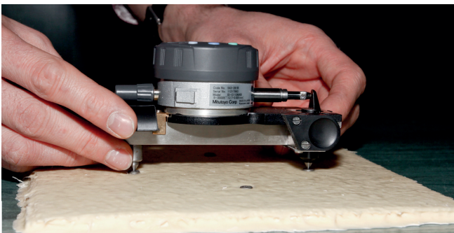
Fig. 5. Extensometer used for length change measurement
