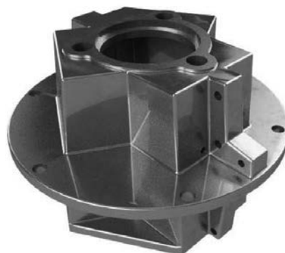
Fig. 2. Disassembled water-lubricated bearing of the Braniewo HEP Plant (on left). Three wooden block compartments and adjusting bolt holes visible. On right computer model of bearing housing
