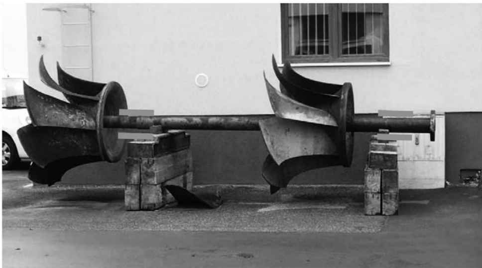
Fig. 1. Disassembled Braniewo HEP Plant turbine shaft with original double Francis turbine arrangement placed one under another. Bottom (subject of analysis – on left) and top (on right) bearing locations marked. In plant shaft operates vertically
