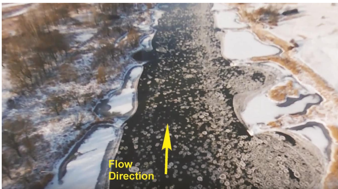
Figure 7. Aerial photograph showing ice movement on 13 January 2017 during windless weather, with an average flow of 150 m 3 /s on the Odra River upstream of Cigacice bend.
