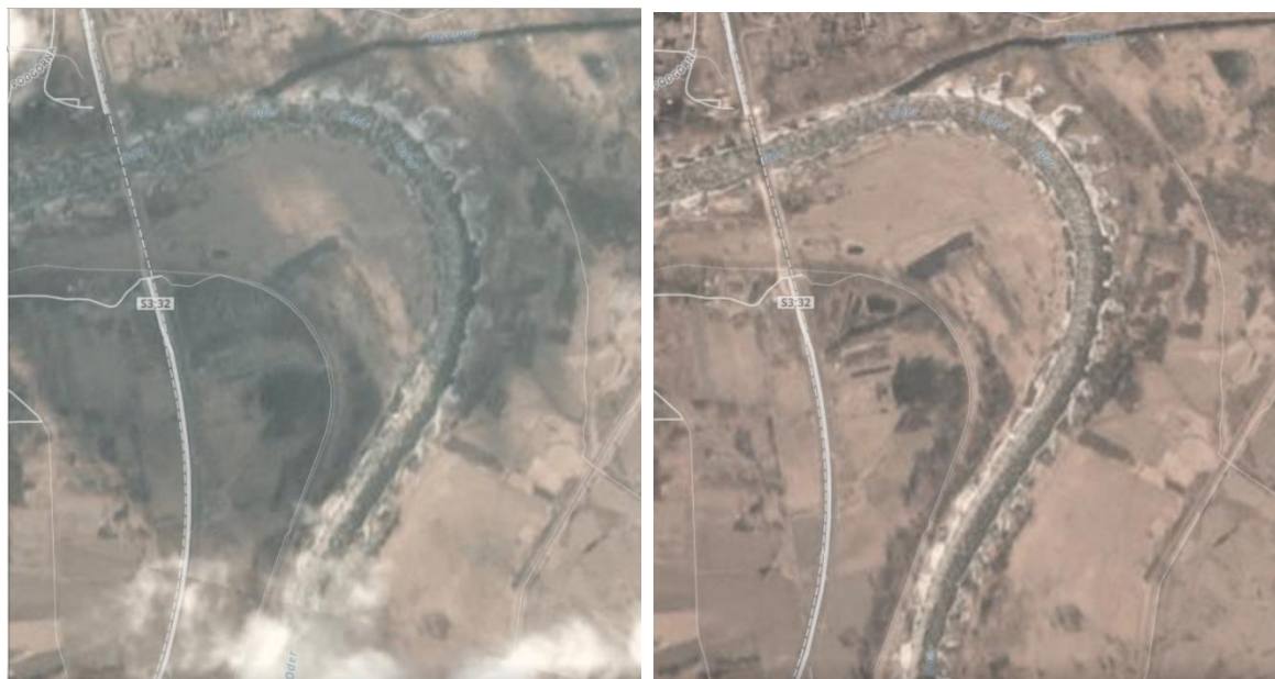
Figure 8. Satellite images (Sentinel 2) of ice movement on the sharp river bend near Cigacice on (a) 28 February and (b) 2 March 2018.
