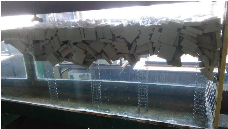
Fig. 4. Ice jam model in GUT hydraulic laboratory, flow direction from left to right
