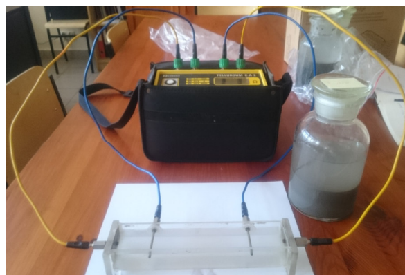
Figure 4. A measuring set used to determine the conductivity of the feed. Digital earth resistance meter, type TELLUROHM C.A 2 and „soil-box” vessel.
