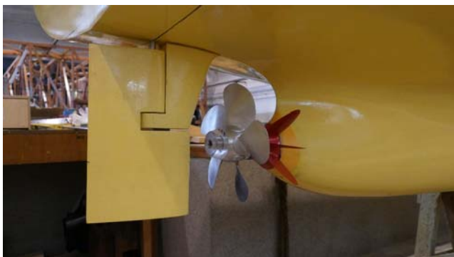
Figure 4. Hull model equipped with propeller CP753 and stator ST002.
