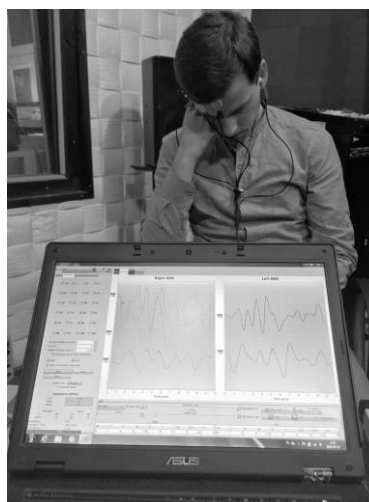
Figure 5. Subject during the preliminary tests - results displayed on the monitor employing a commercial ABR software interface [6]
