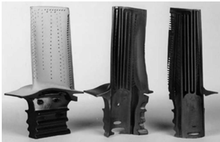
Figure 11: Gas turbine blades with cooling holes (left).
