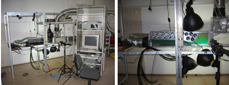
Figure 7: The view of test rig: wind tunnel and data acquisition system (left), test section and lighting system (right).
