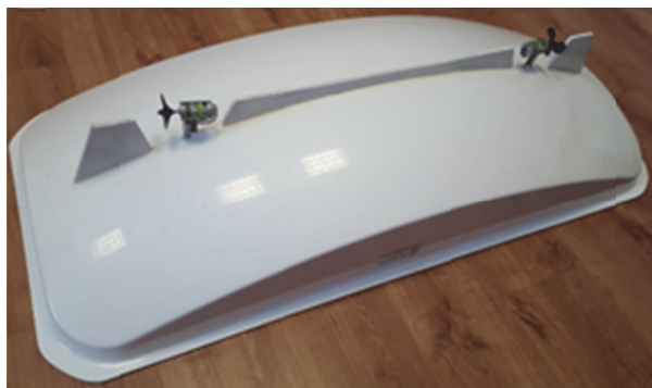
Fig. 2 The final version of 1:10 scale model with skegs and azimuth thruster.
