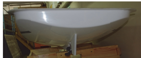
Fig. 8 Front view of the model with appendages
