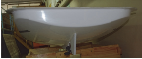
Fig. 10 Model with appendages during the test
