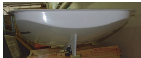
Fig. 9 Model without appendages during the test
