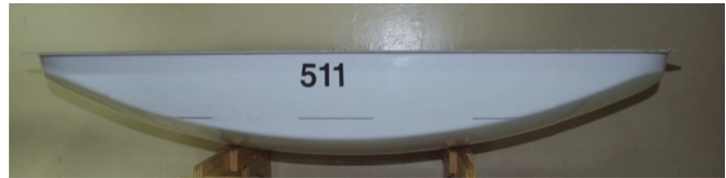
Fig. 5 Side view of the model without appendages
