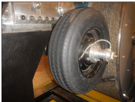
Figure 3: Roadwheel facility with 2.0 m diameter drum at the Technical University of Gdańsk, Poland
