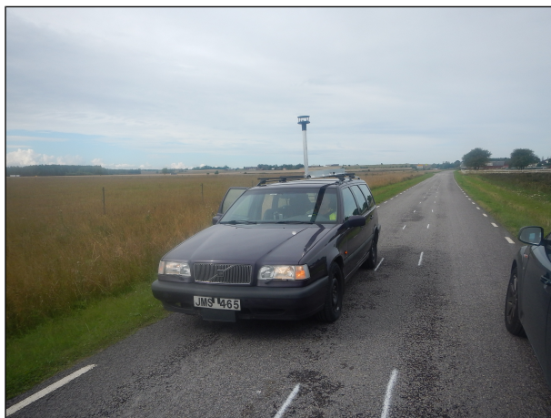
Figure 5: Car equipped for coast-down measurements of rolling resistance
