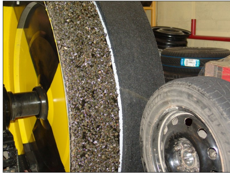
Figure 4: Testing of rolling resistance of passenger car tire on Rosehill PERS at TUG
