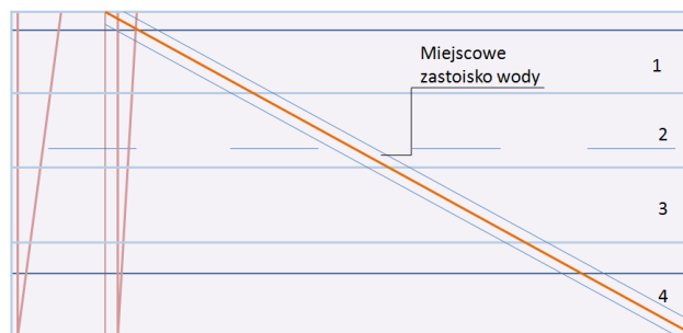
Fig. 8. The approved method for dividing the road works zone into 4 working plots ("Miejscowe zastoisiko wody" (pol.) = the ponding of water).
