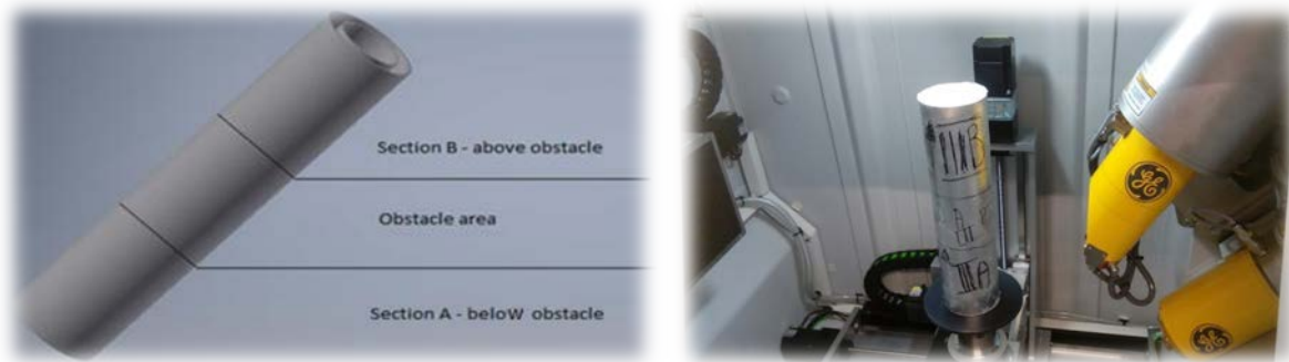
Fig. 8. Section cuts schematic drawings and a specimen inside the scanner
