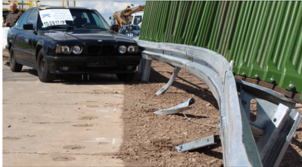
Fig. 4 Steel road safety barrier N2/W4/A after exemplary crash test
