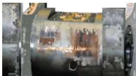
Fig. 5. Image of the damaged surface of crosshead pin resulting from an excessive wear due to friction and corrosion [30]
