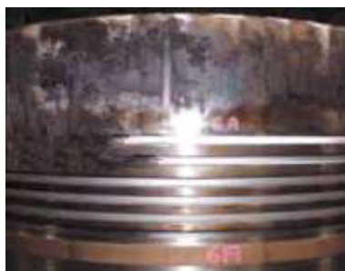
Fig. 3. Image of a piston damaged due to excessive friction wear of piston ring surface and significant damage of piston rings [30]
