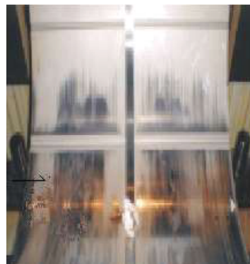
Fig. 6. Image of the damaged surface of sliding coat of crank-end bearing sleeve due to its excessive friction wear [30]
