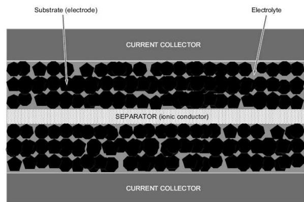
Fig.1. Schematic diagram of symmetric supercapacitor [1]
