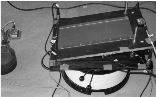
Fig. 4. System of the sensors for testing the range of the platform movement mounted to the oscillating device
