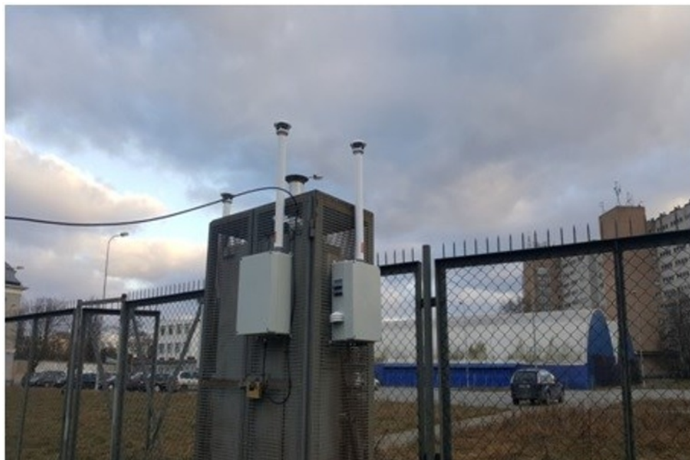
Fig. 1. PM10 sensors (white box) mounted on the protective case of the reference station located in Gdańsk, Poland.
