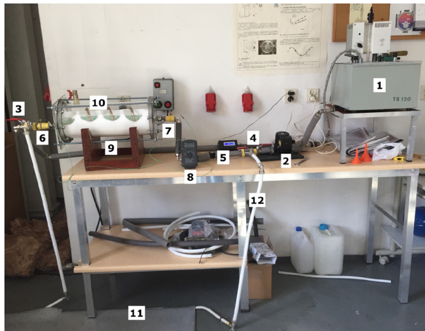
Fig. 1. View of the experimental stand; 1 – thermostat; 2 – circulator pump; 3,4 – set of valves; 5 – flowmeter; 6, 7 – thermocouples; 8 – temperature recorder; 9, 10 – LHTE filled with PCM, 11, 12 – tap water system
