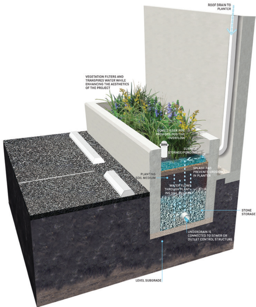
Fig. 10. Flow-Through Planter Box with Typical Features (source: [18])
