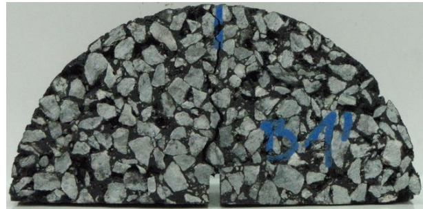
Fig. 4. Porous asphalt PA 8
