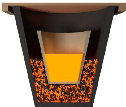
Figure 1: A schematic view of a double crucible technique. The inner crucible contains the batch. The outer crucible is half-filled with activated charcoal and covered with a lid. At elevated temperatures activated charcoal bonds with oxygen creating \text{CO} , which is a reducing agent.
