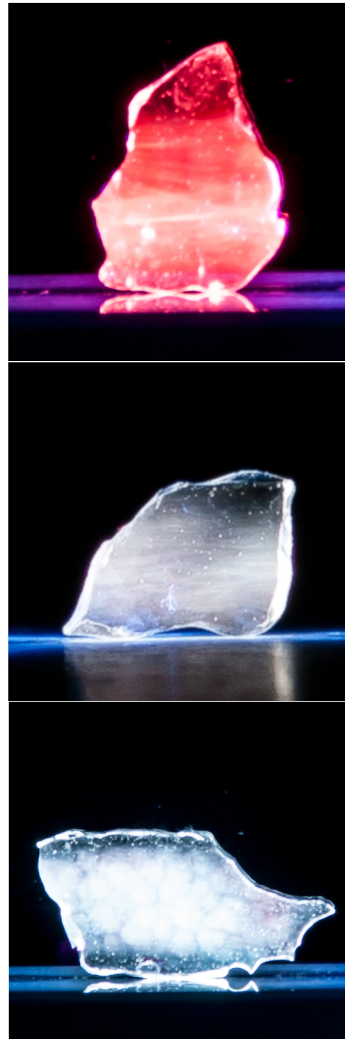
Figure 6: Photographs of photoluminescence of samples A (top), B (middle) and C (bottom) excited by a blue laser diode. The samples are ca. 1 cm high.
