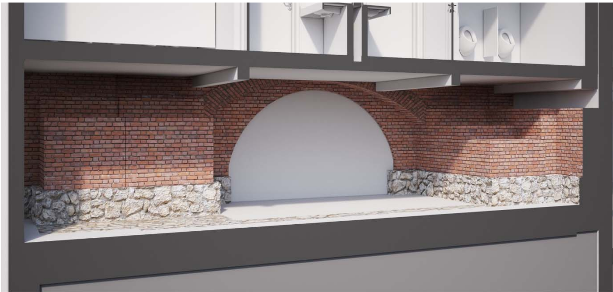
Figure 3. The concept of adaptation, along with the reconstruction, of the towers foundations in the planned space of the Gateway Passage building (source: Author's Jacek Bułat Architectural Studio)
