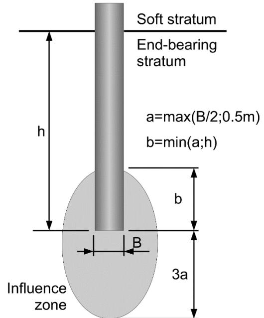
**Fig. 1.** Model for equivalent cone resistance ( $q_{ce}$ ) determination.
