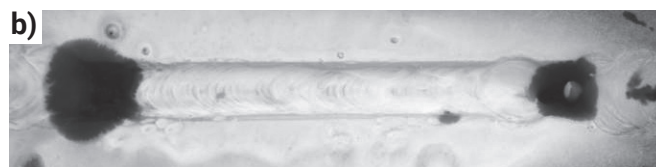
Fig. 5. Results of non-destructive testing for specimen P2, welded in the air, a) VT – crack in the crater, b) PT – crack in the crater
